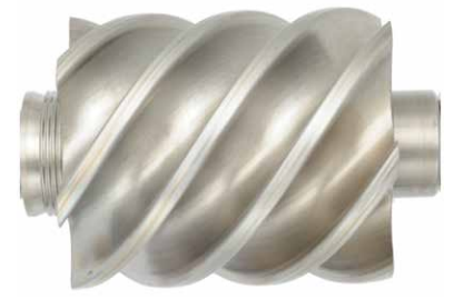
Mobil SHC™ Rarus after 2,640 hours of testing
